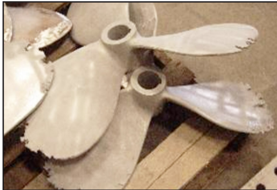
Severely abraded stainless steel agitators
