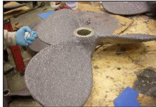
Applying ARC BX2* being applied to the agitator
